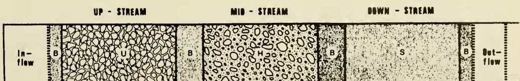
Fig. 1. Schematic diagram of an artificial channel showing the stream sections and one cobble-embeddedness arrangement: (U) = unembedded cobbles, (H) = 50%-embedded cobbles, (S) = 100%-embedded cobbles, and (B) = sand buffer zones.
